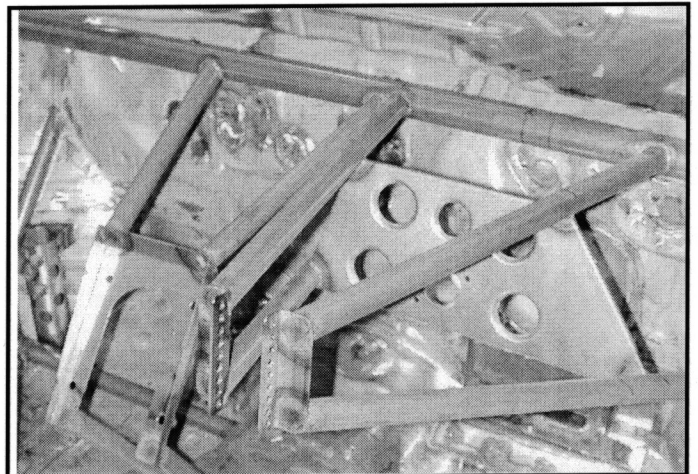
PHOTO N° 34 Steering column support
